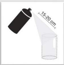
Apply AESUB white from 15-20 cm away. Spray over the entire surface that you will be scanning. Gently push down the spray button and move the can across the area using even, back and forth strokes. Move at a consistent pace without pausing at one point to achieve an even coat. Once the coat is applied, you can scan the object in usual manner.
